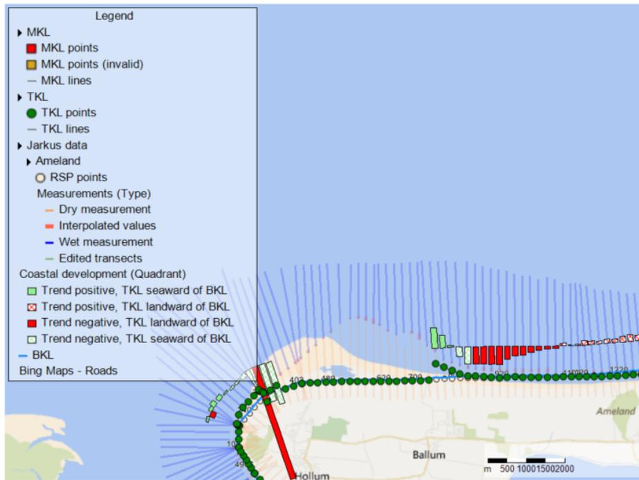
**Figure 7.7:** Typical development overview screen showing results from the coastal development model. The Time Navigator window can be seen below the map.
