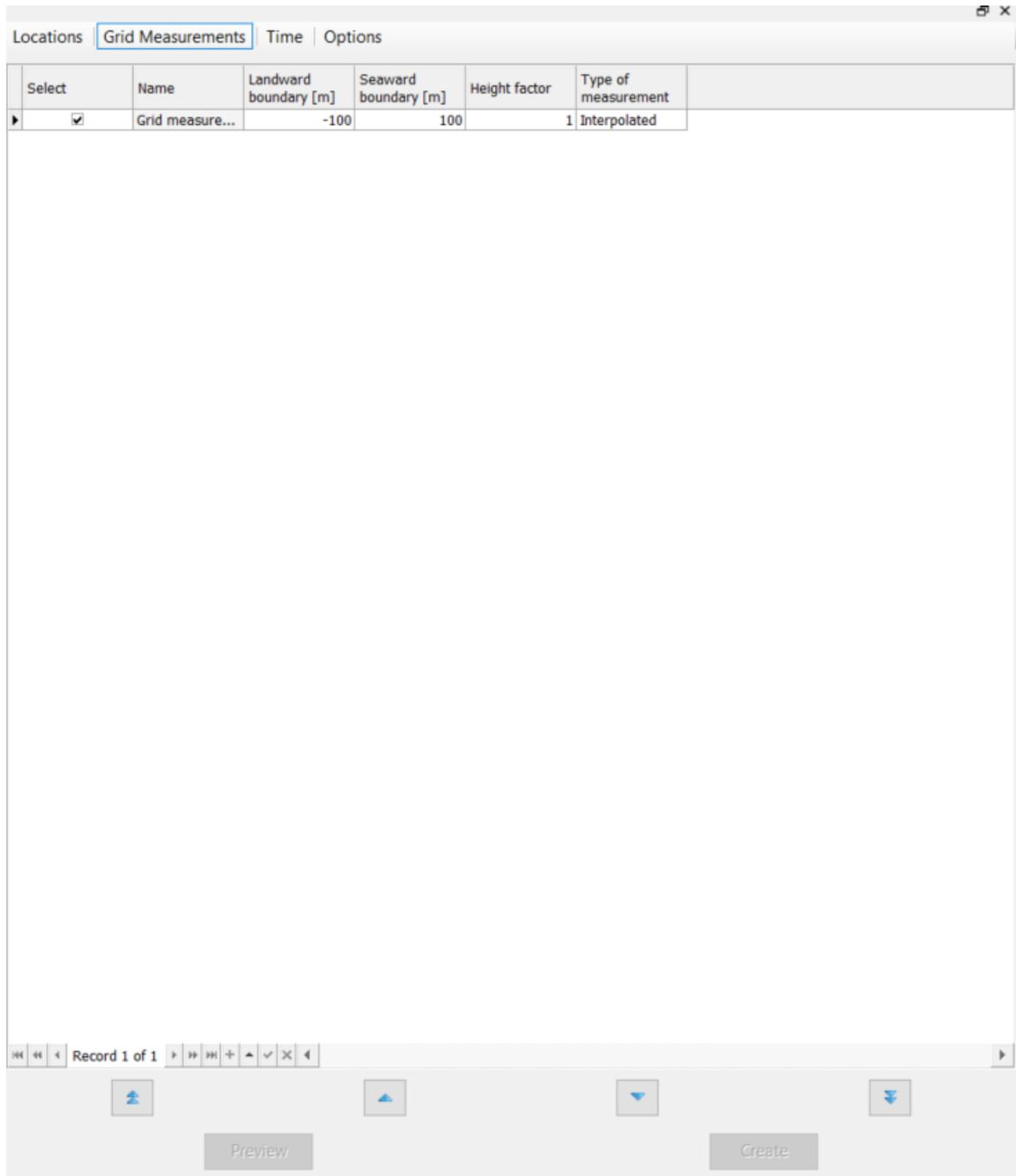
**Figure 5.27:** Grid measurement selection panel for generation of intermediate transects
