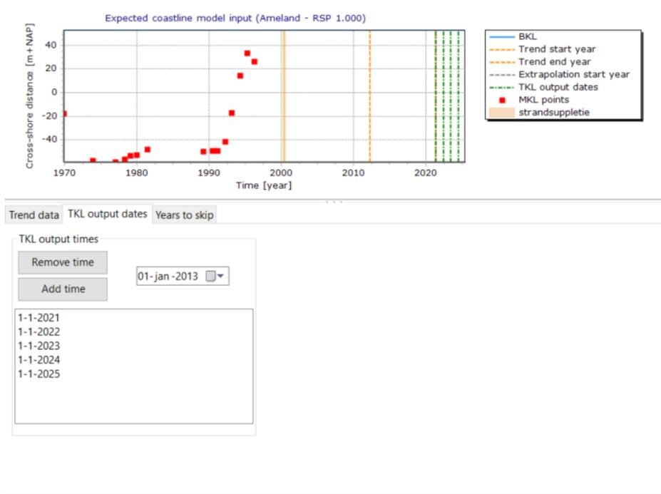
Figure 7.4: Typical window for defining output dates for calculating TKL values.
