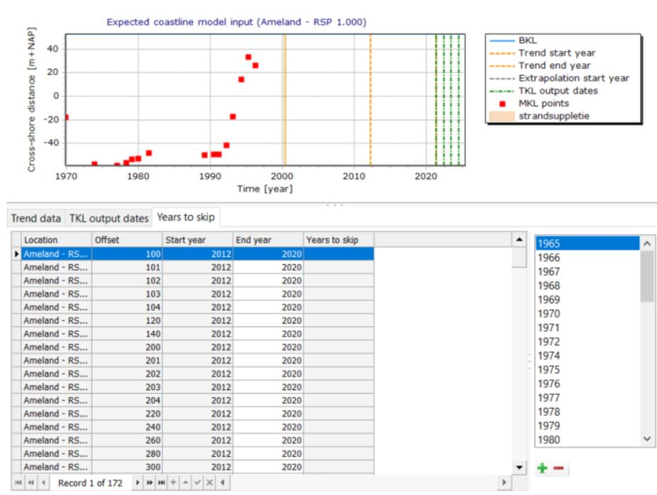
*Figure 7.5: Typical window for specifying years to skip during calculation*
