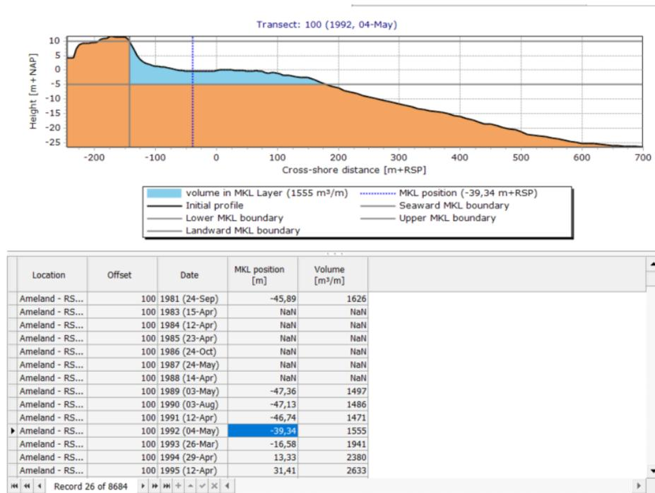
Figure 7.1: Typical screen showing calculated MKL points
