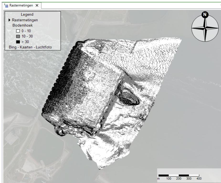
**Figure 4.11:** Typical map display of the calculated slopes.
