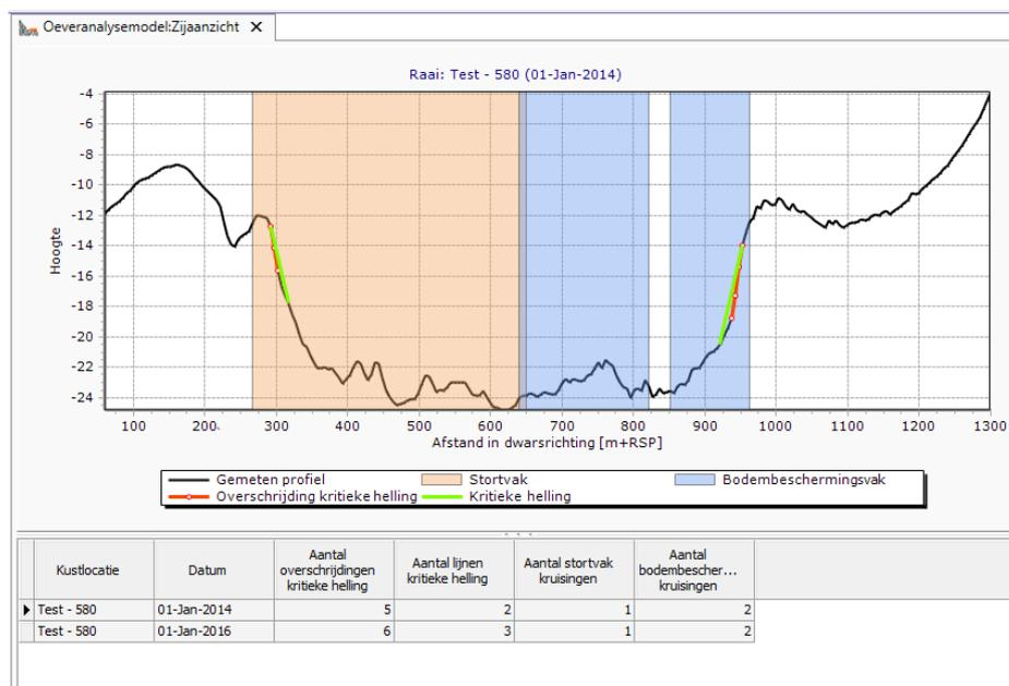
Figure 9.6: Side view of a profile measurement in the bank analysis model.
