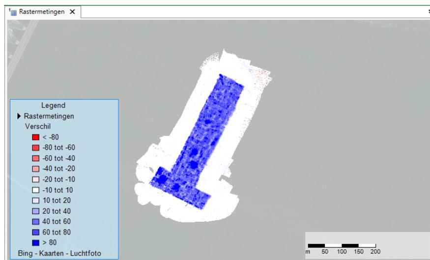
**Figure 4.14:** Visualization of the difference in bed height due to a nourishment
