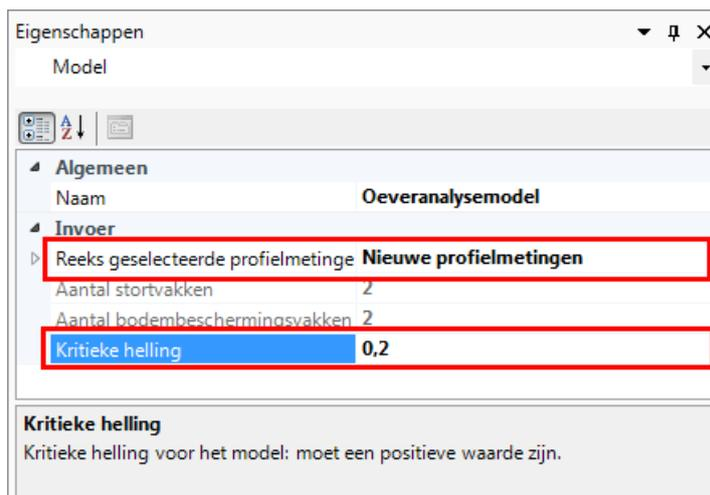
Figure 9.2: Properties of a bank analysis model
