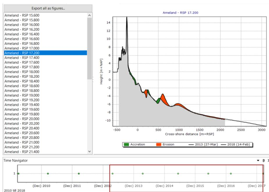
**Figure 4.7:** Typical Time difference visualization showing also the Time Navigator setting of the analysis period.
