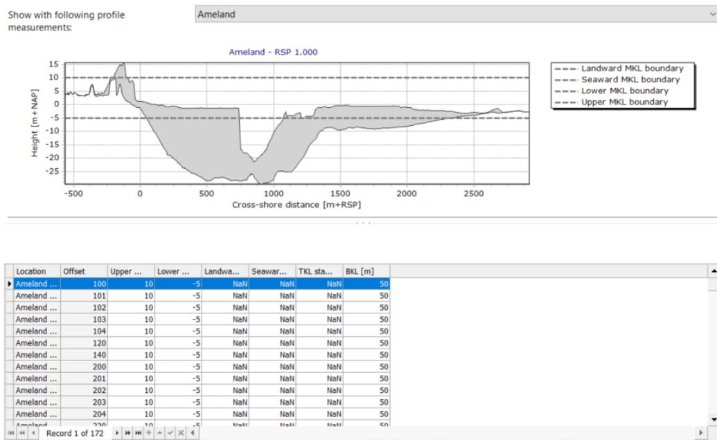
Figure 5.8: Document window showing (lower section) boundary conditions table and (upper section) corresponding figure of profile measurements and vertical boundaries from the boundary conditions.
