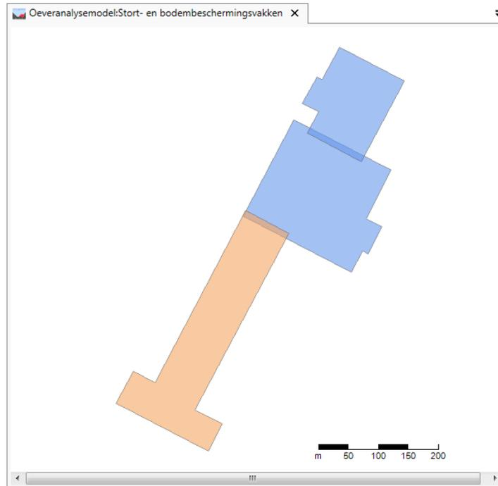
**Figure 9.4:** Plan view of landfill (orange) and two bottom protection areas (blue).
