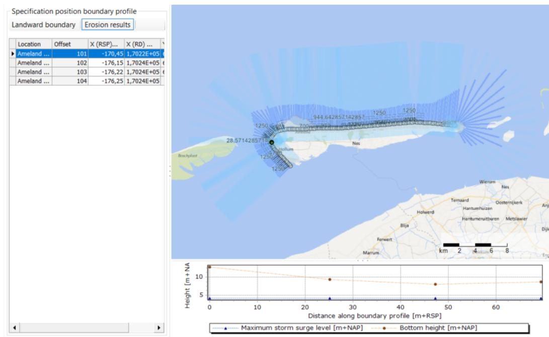
**Figure 6.6:** Typical document window showing plan view geometry for boundary profile design
