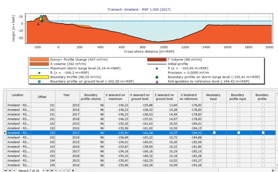
**Figure 6.10:** Typical boundary profile screen showing results of a modeling run
