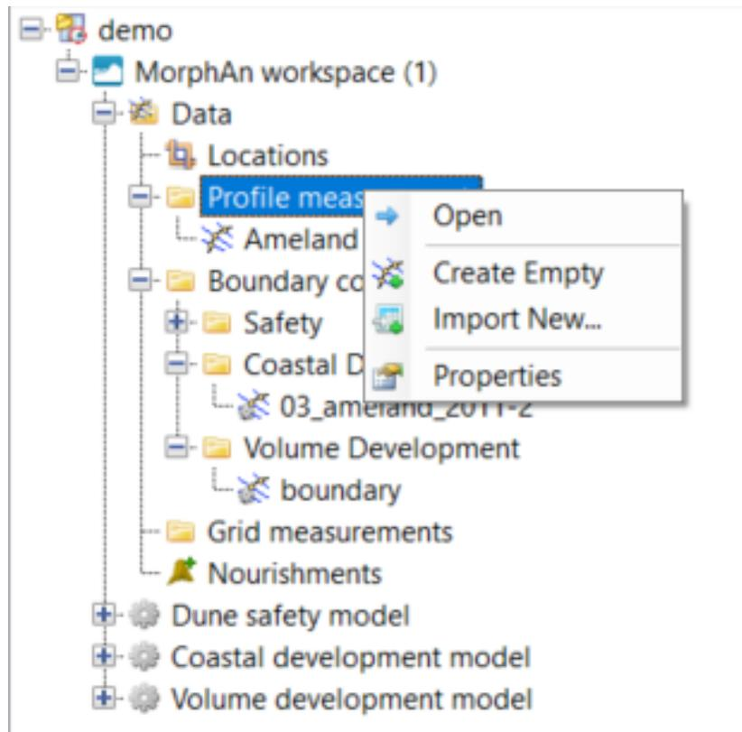
**Figure 3.15:** Menu for managing profile measurements within a workspace
