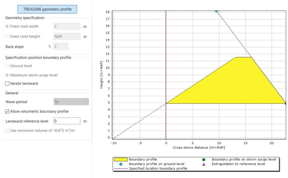
Figure 6.9: Typical cross-shore geometry window in the boundary profile model
