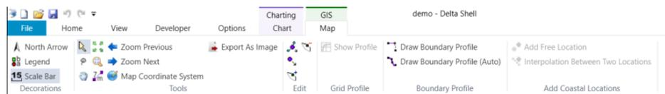
**Figure 6.8:** The Map Ribbon tab, showing the tools that are useful for boundary profile design circled in red
