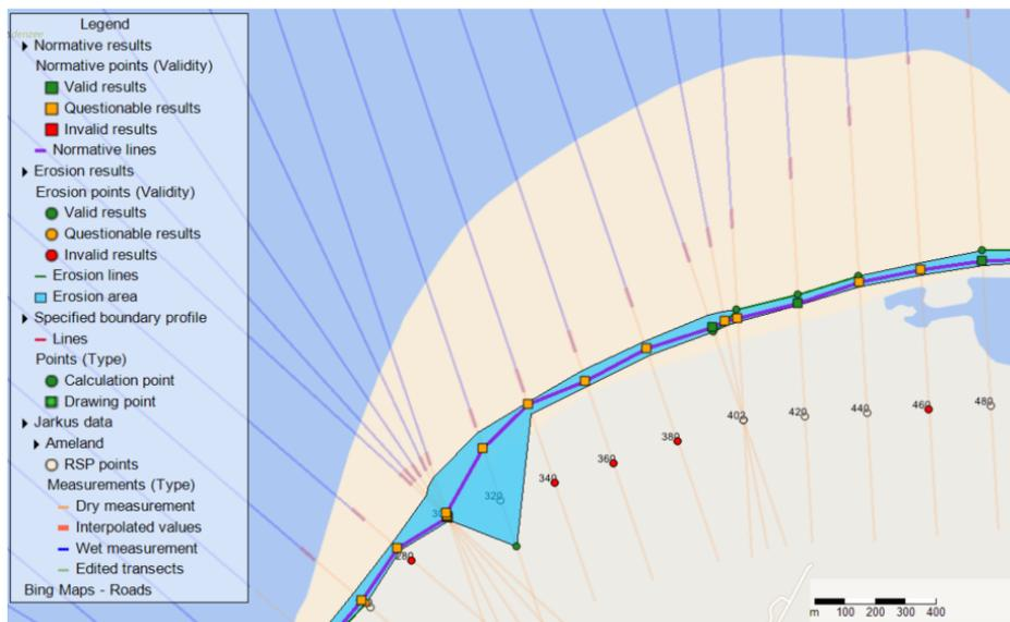
Figure 6.14: Typical Dune safety overview window showing results of a modeling run for Vlieland
